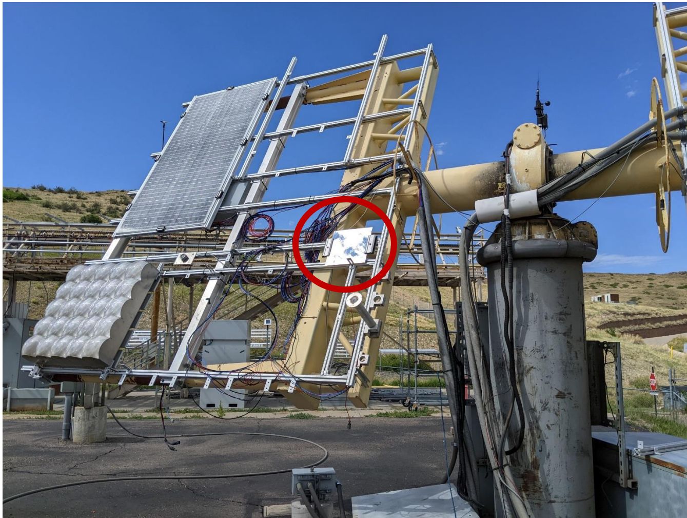
Configurable solar tracker at the NREL Outdoor Test Facility
